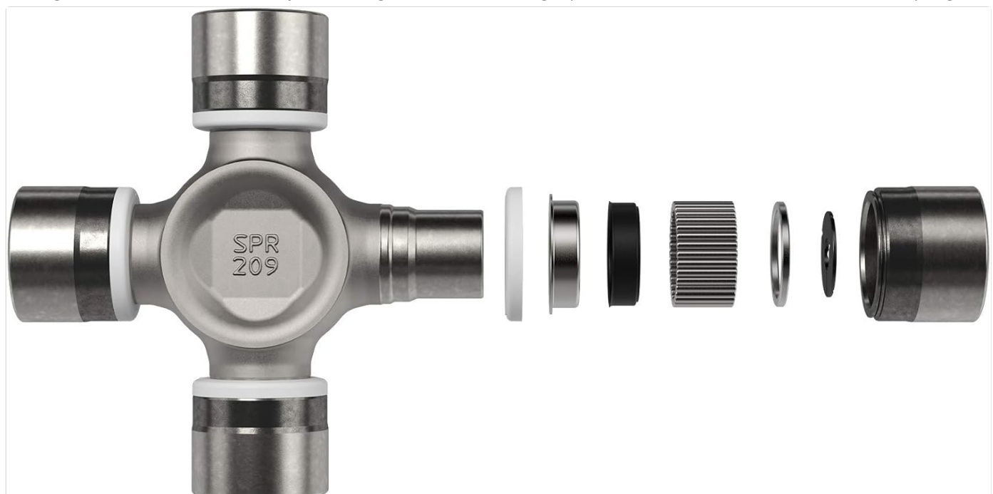
Image: Exploded view illustrating the individual components of the Spicer U-Joint, including the cross, bearing cups, seals, and thrust
