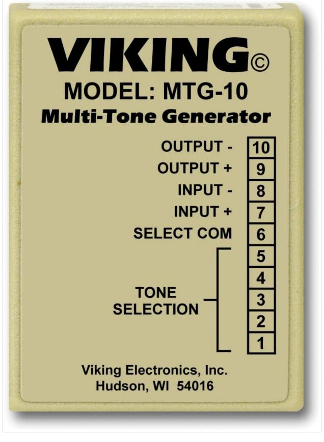
This image displays the product label for the VIKING MTG-10 Multi-Tone Generator. The label clearly indicates the wiring terminals: OUTPUT - (pin 10), OUTPUT + (pin 9), INPUT - (pin 8), INPUT + (pin 7), and SELECT COM (pin 6). Below these, pins 1 through 5 are designated for 'TONE SELECTION'. The label also includes the manufacturer's name and address: Viking Electronics, Inc., Hudson, WI 54016.
