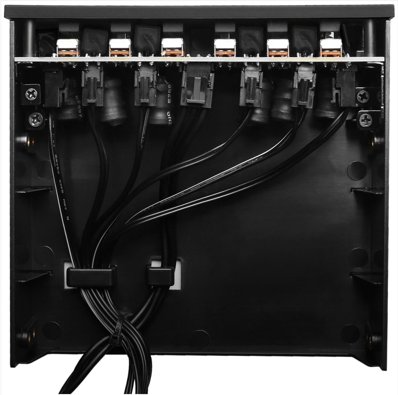
Figure 2: Rear view of the NZXT Sentry Mix 2 Fan Controller, showing the six fan headers with cables connected. This image demonstrates how fans are plugged into the controller's output ports.
