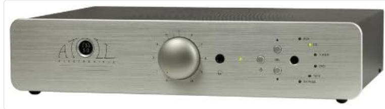
Front view of the ATOLL IN50SE integrated amplifier, showing the central volume knob, input selection buttons, and power indicator.
