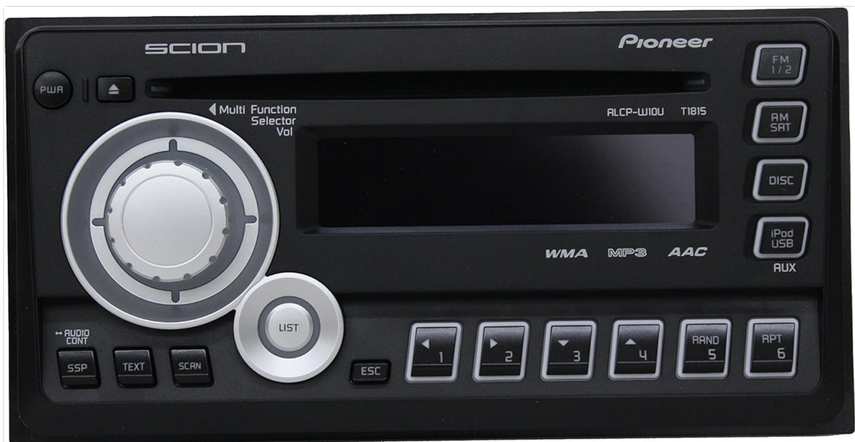
Figure 2: Front panel of the audio system, highlighting the power button, multi-function selector, display, and various source/preset buttons.
