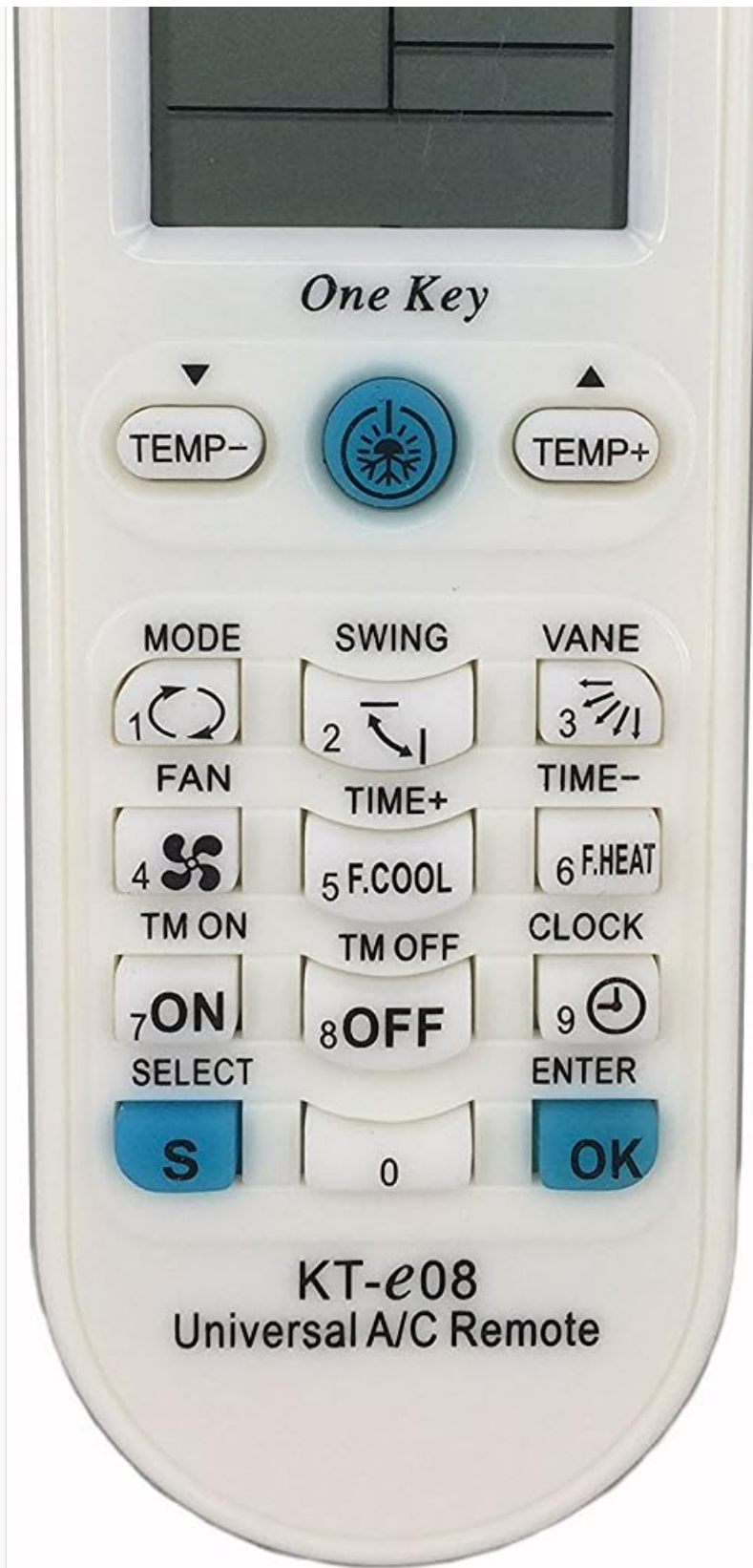
Figure 1: KT-E08 Universal A/C Remote Control. This image displays the remote's layout, including the LCD screen, temperature buttons, mode, fan, swing, vane, timer, and numeric keys.
