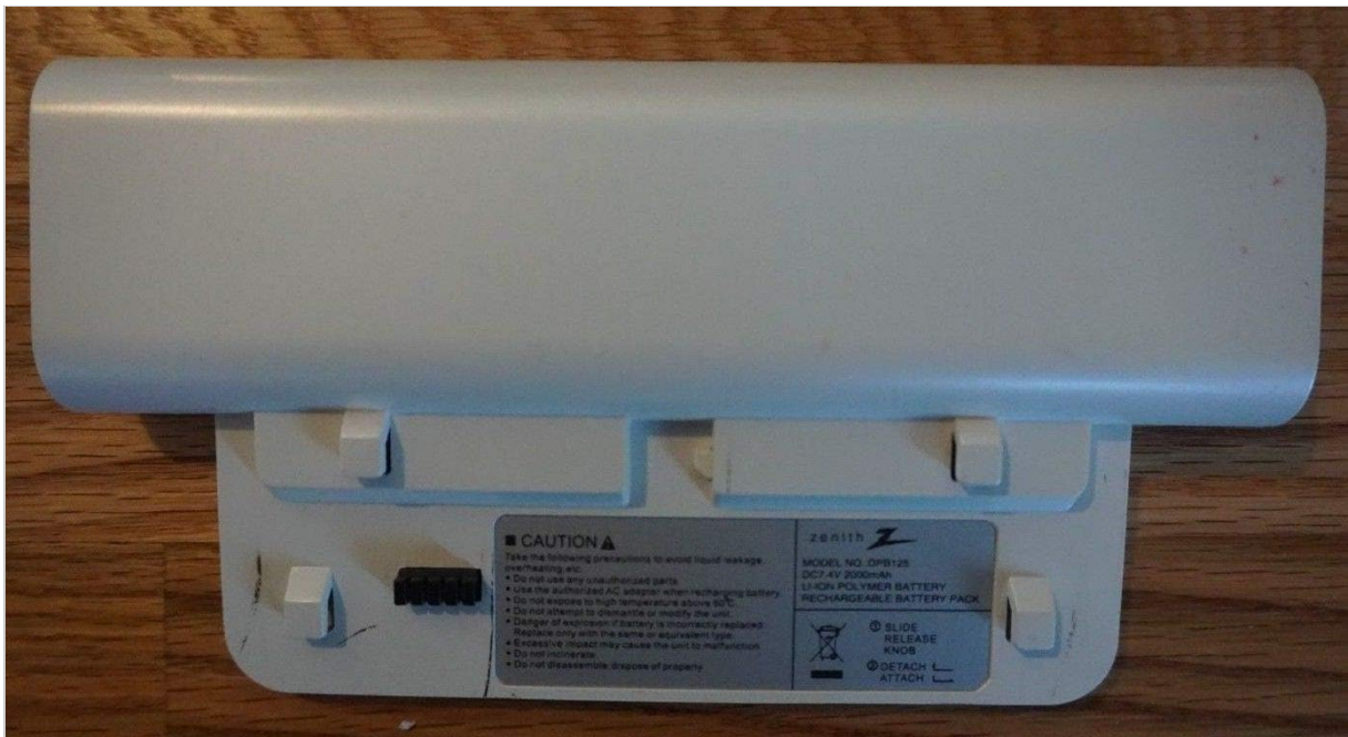
Figure 4.5: Top view of the Zenith rechargeable battery pack (Model SPB125), showing its specifications (DC 7.4V 2000mAh) and caution labels regarding proper use and disposal.
