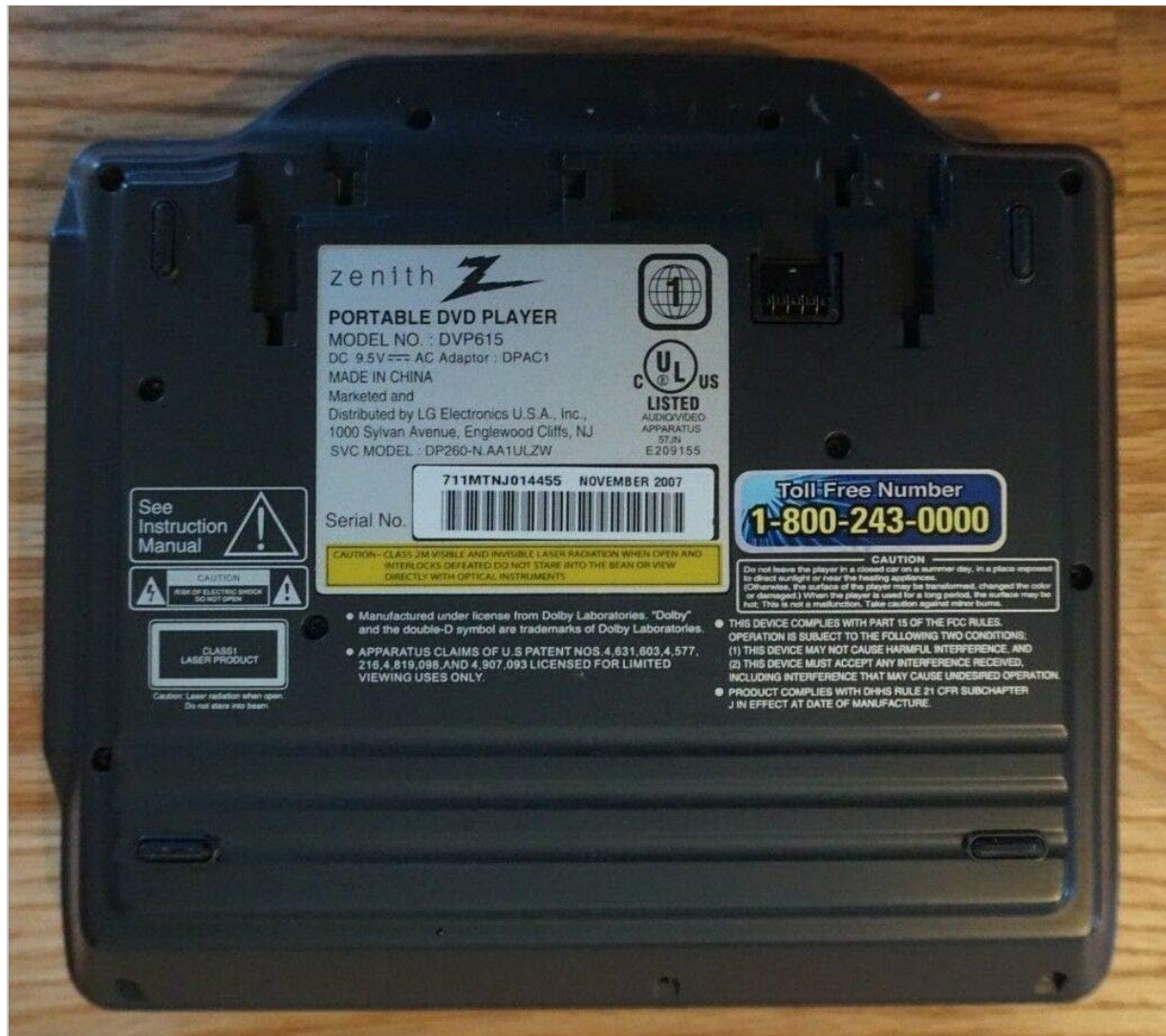
Figure 9.1: Bottom view of the Zenith DVP615 Portable DVD Player, showing the product label with model number DVP615, serial number, power requirements (DC 9.5V AC Adaptor), and manufacturing details.
