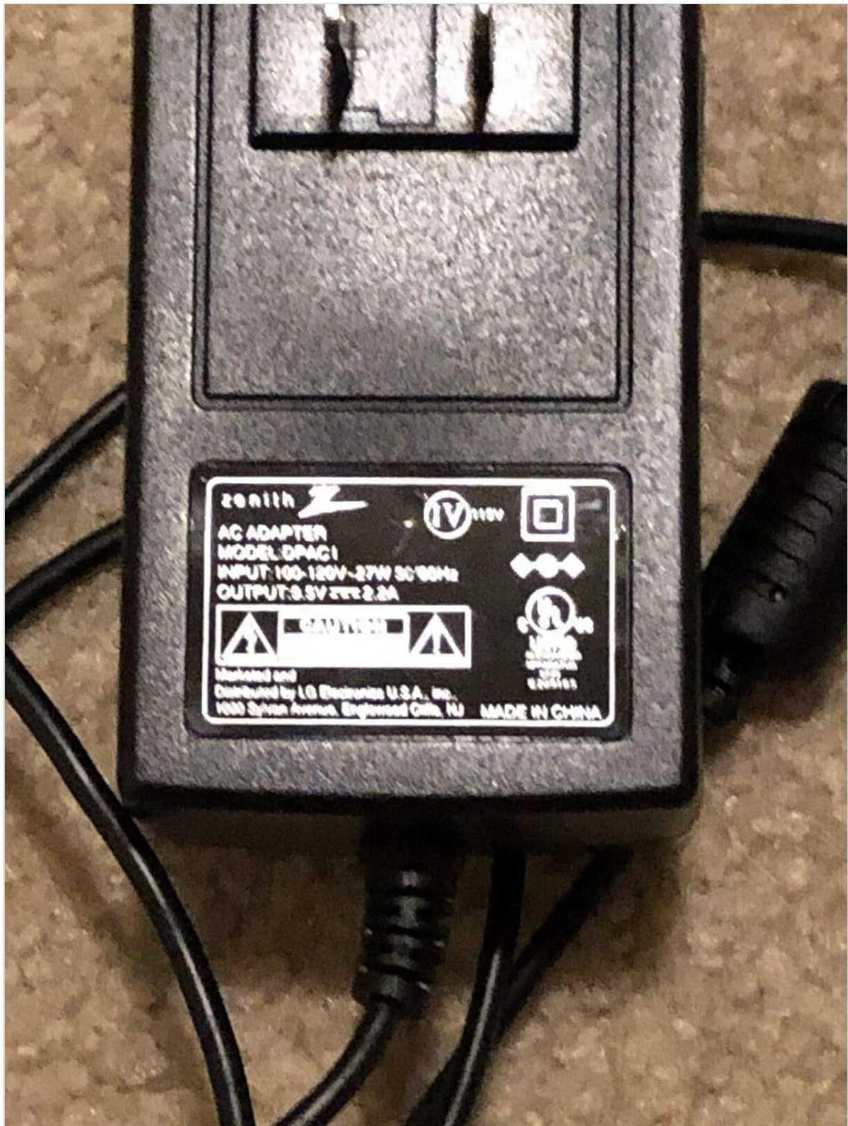
Figure 4.4: Close-up of the Zenith AC adapter (Model DPAC1), showing input (100-120V~27W 50/60Hz) and output (9.5V \approx 2.5A) specifications.
