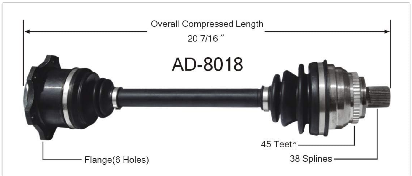
Figure 2: Dimensional drawing of the AD-8018 CV Axle Shaft, illustrating key measurements such as overall compressed length, flange hole count, and spline/teeth counts.
