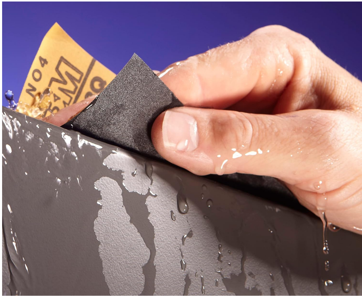
Figure 3: A hand demonstrating the wet sanding process using a piece of the 3M Wetordry Abrasive Sheet on a grey surface, with water visibly flowing over the area to facilitate the sanding action.
