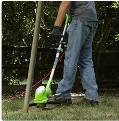
Figure 3: The trimmer head rotated 180 degrees for edging functionality.
