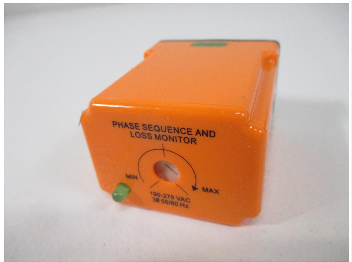
Figure 2: Front view of the SLA-230-ASA showing the adjustment dial.
