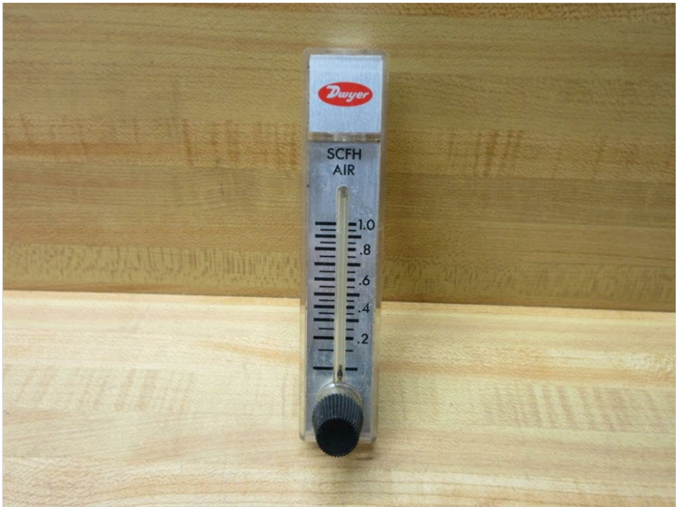
Figure 2: Front view of the Dwyer Rate-Master Flowmeter, highlighting the SCFH AIR scale and the integrated adjustment knob for precise flow control.
