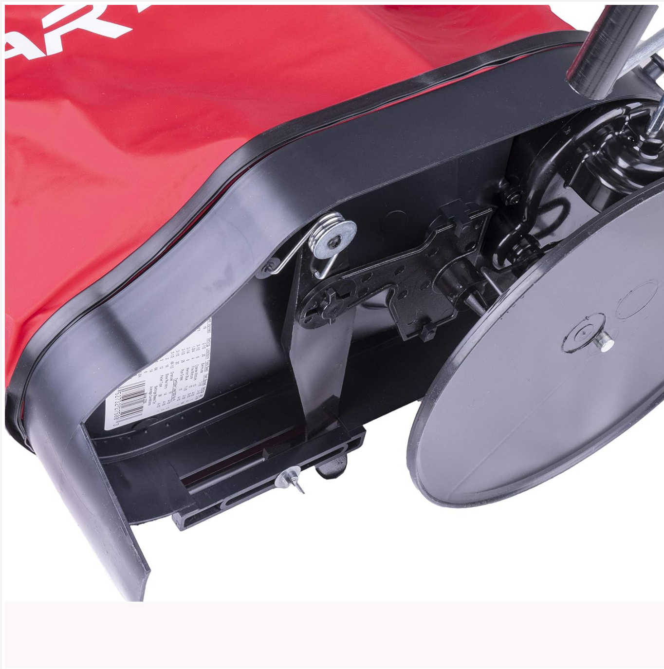
Figure 6: Underside view of the spreader's broadcast mechanism.
