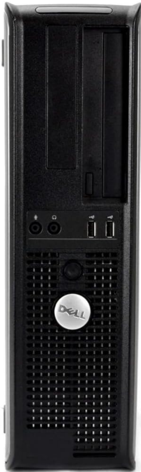
Image: Front view of the Dell Optiplex 755 SFF, showing the optical drive bay and front panel connections.
