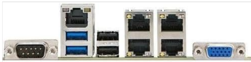
Figure 2.3: Rear I/O panel of the Supermicro X10SLM+-LN4F motherboard, featuring multiple LAN ports, USB ports, and serial ports.
