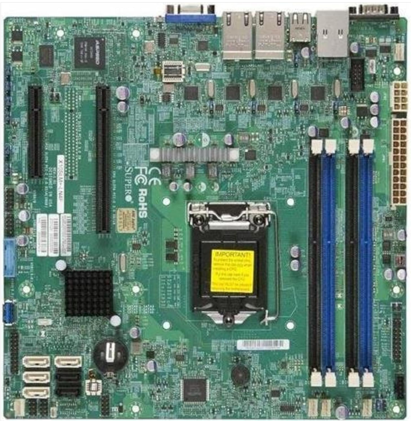
Figure 2.1: Top-down view of the Supermicro X10SLM+-LN4F motherboard, showing the CPU socket, DIMM slots, PCIe slots, and various connectors.
