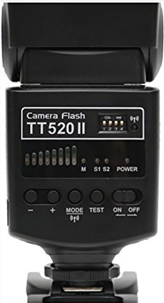
Figure 2: Detailed view of the flash control panel, showing mode, power, and test buttons.
