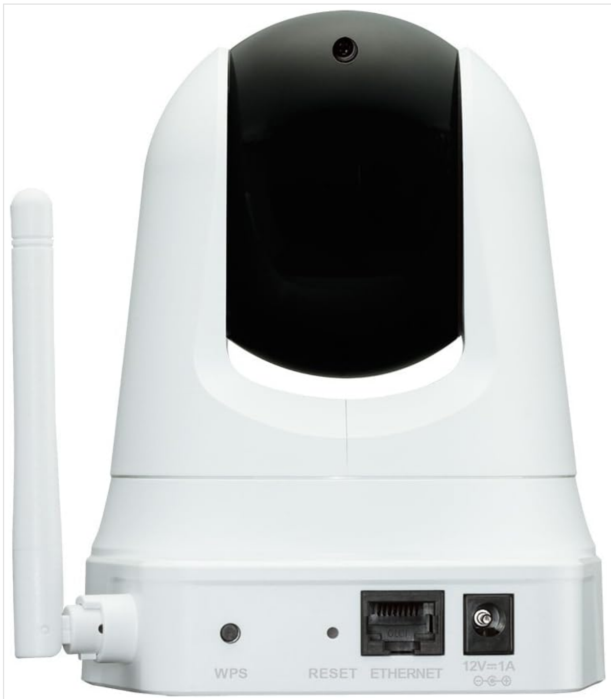
Figure 3.3: Rear view of the D-Link DCS-5020L camera, highlighting the WPS button, Reset button, Ethernet port, and 12V=1A power input.
