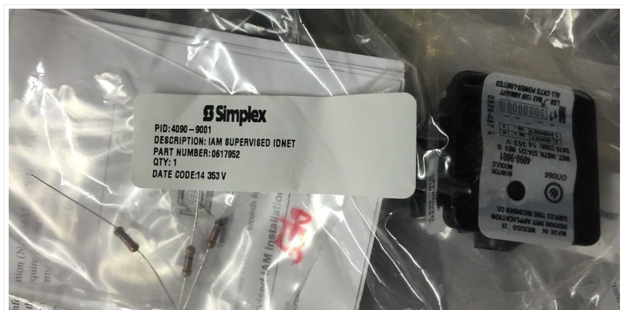
Figure 3.2: The Simplex 4090-9001 module shown within its clear plastic packaging. The packaging includes a label with "PID: 4090-9001", "DESCRIPTION: IAM SUPERVISED IDNET", and "PART NUMBER: 0617952". Small resistors are also visible in the package.
