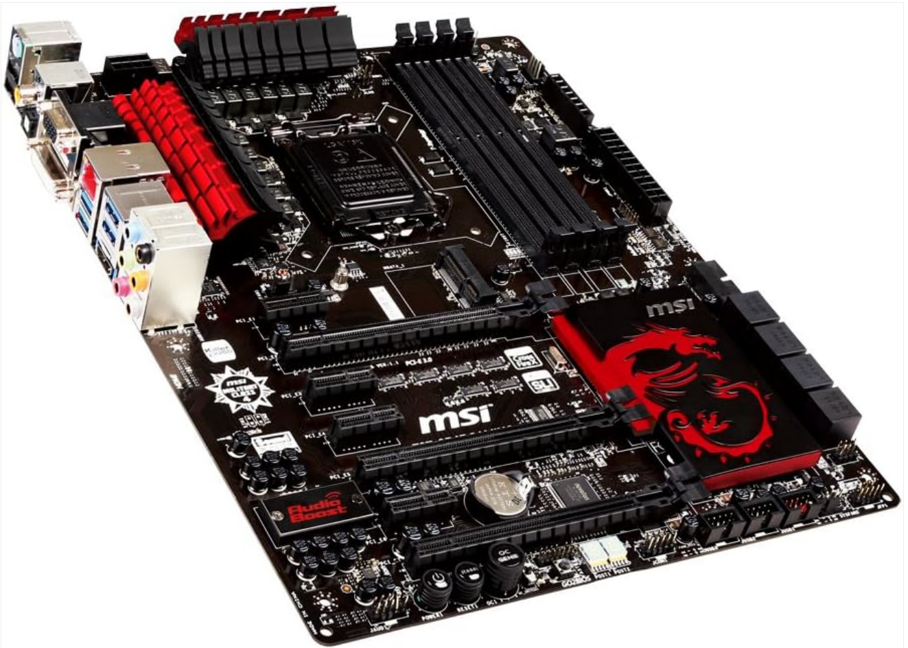
Figure 2.2.1: Angled view of the MSI Z87-G45 GAMING motherboard, showcasing the heatsinks, expansion slots, and various connectors.
