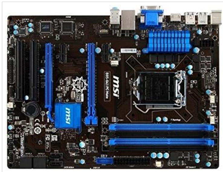
Figure 7.1: Rear I/O panel of the MSI B85-G41 PC Mate Motherboard, showing various connectivity ports.
