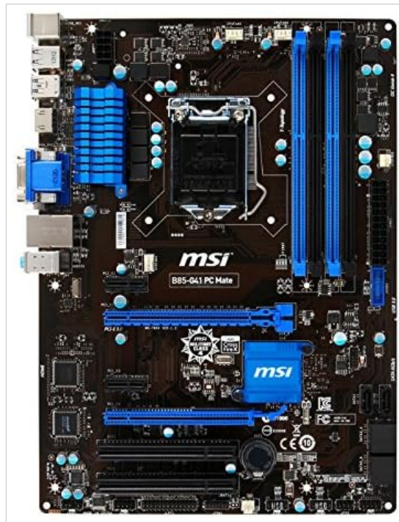
Figure 2.2: Angled view of the MSI B85-G41 PC Mate Motherboard, showing the heatsinks and various connectors.
