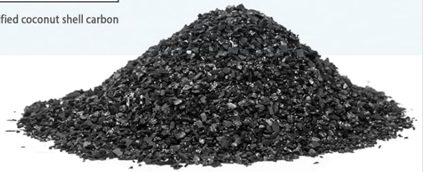
Figure 3: Illustration of the coconut shell granular activated carbon media, highlighting its effectiveness in removing soil, taste, odors, chlorine, and sediment.
