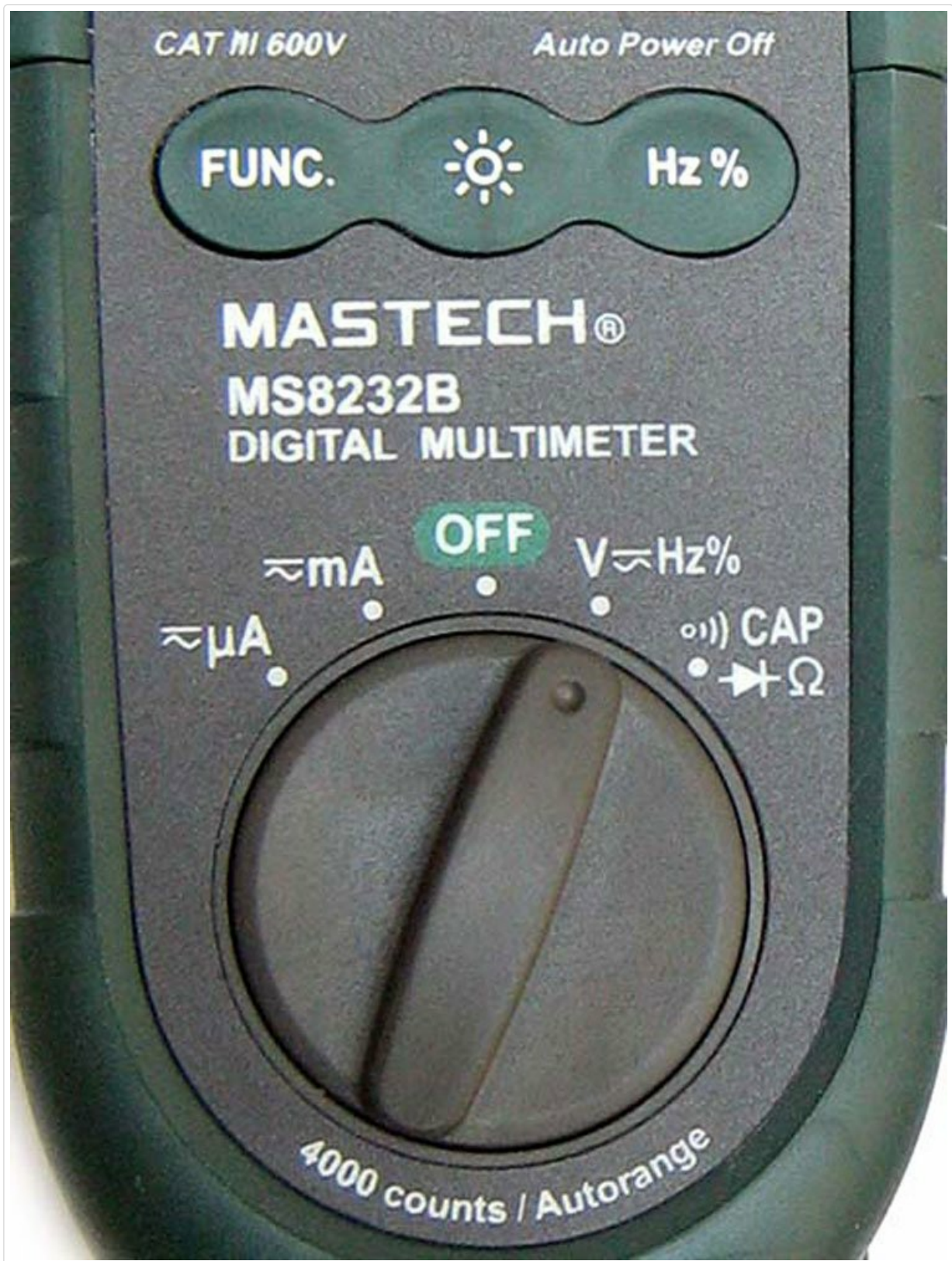
Figure 3.2: Close-up of the rotary switch and function buttons, including FUNC, Flashlight, and Hz%.
