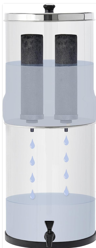
Image 6.2: A diagram showing how water flows from the upper chamber, through the Black Berkey Elements, and collects as filtered water in the lower chamber. Key contaminants removed are listed.
