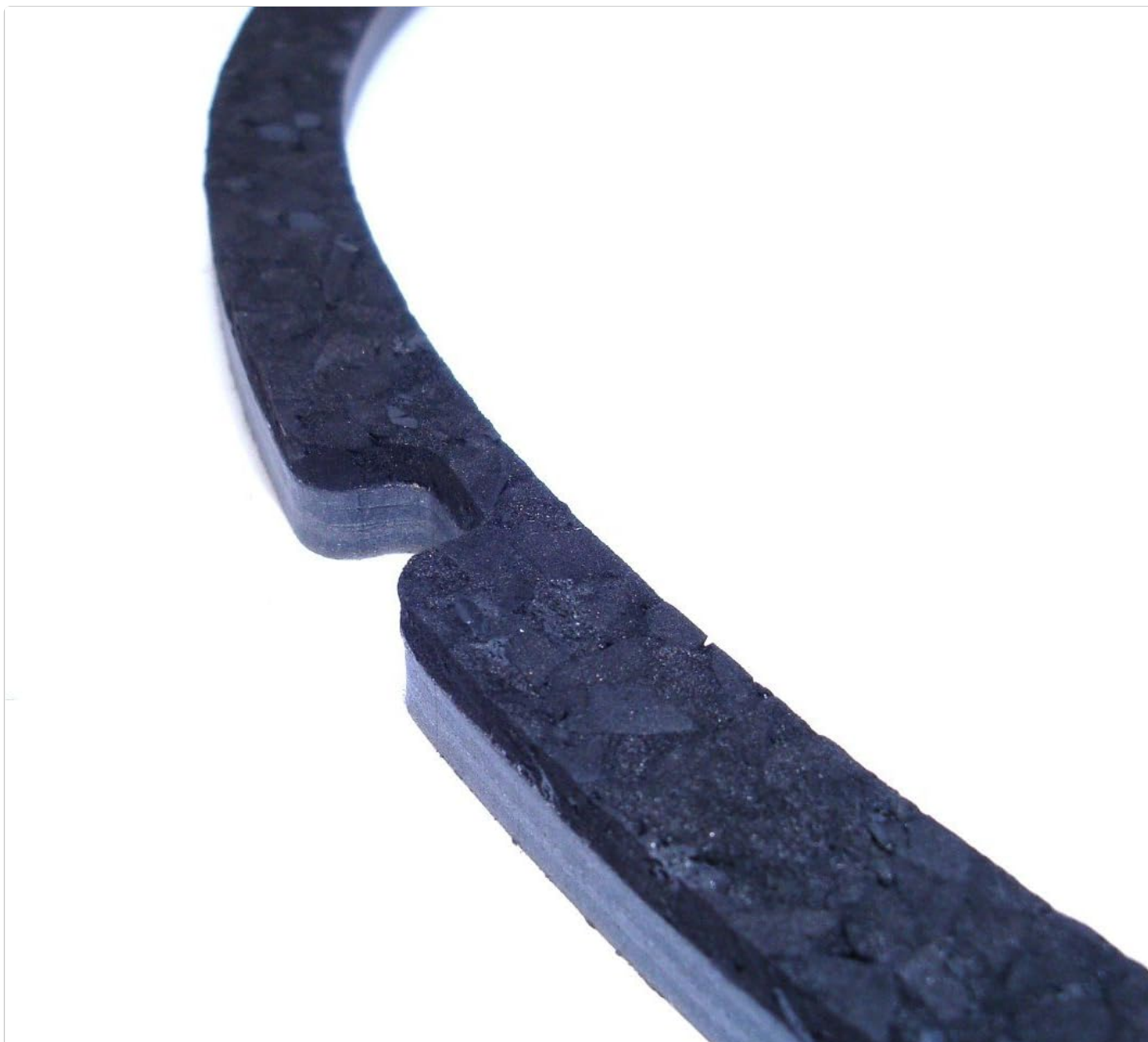
Image 1.2: Close-up view of the Rubitex gasket material, illustrating the laminated construction of Rubitex and Chip layers.
