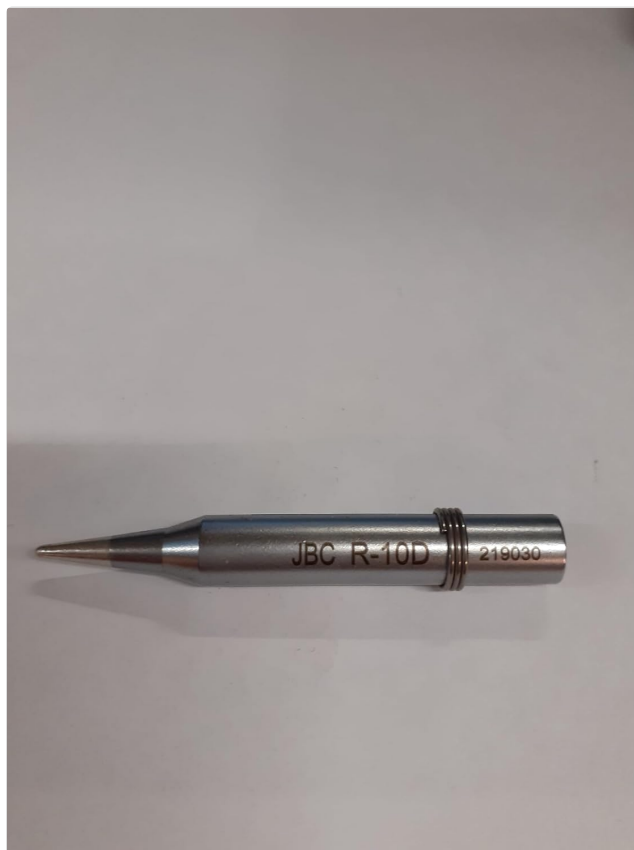
Image 1: The JBC R10D soldering tip, showing its conical shape and the engraved model number.
