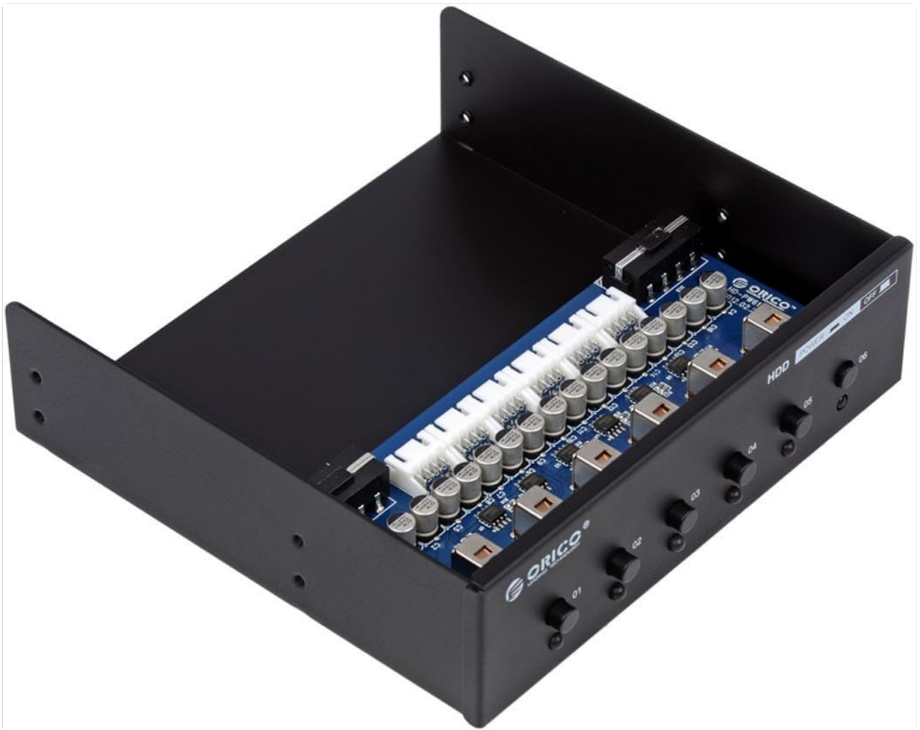
Figure 5: Internal view of the ORICO HD-PW6101 with SATA output connectors.
