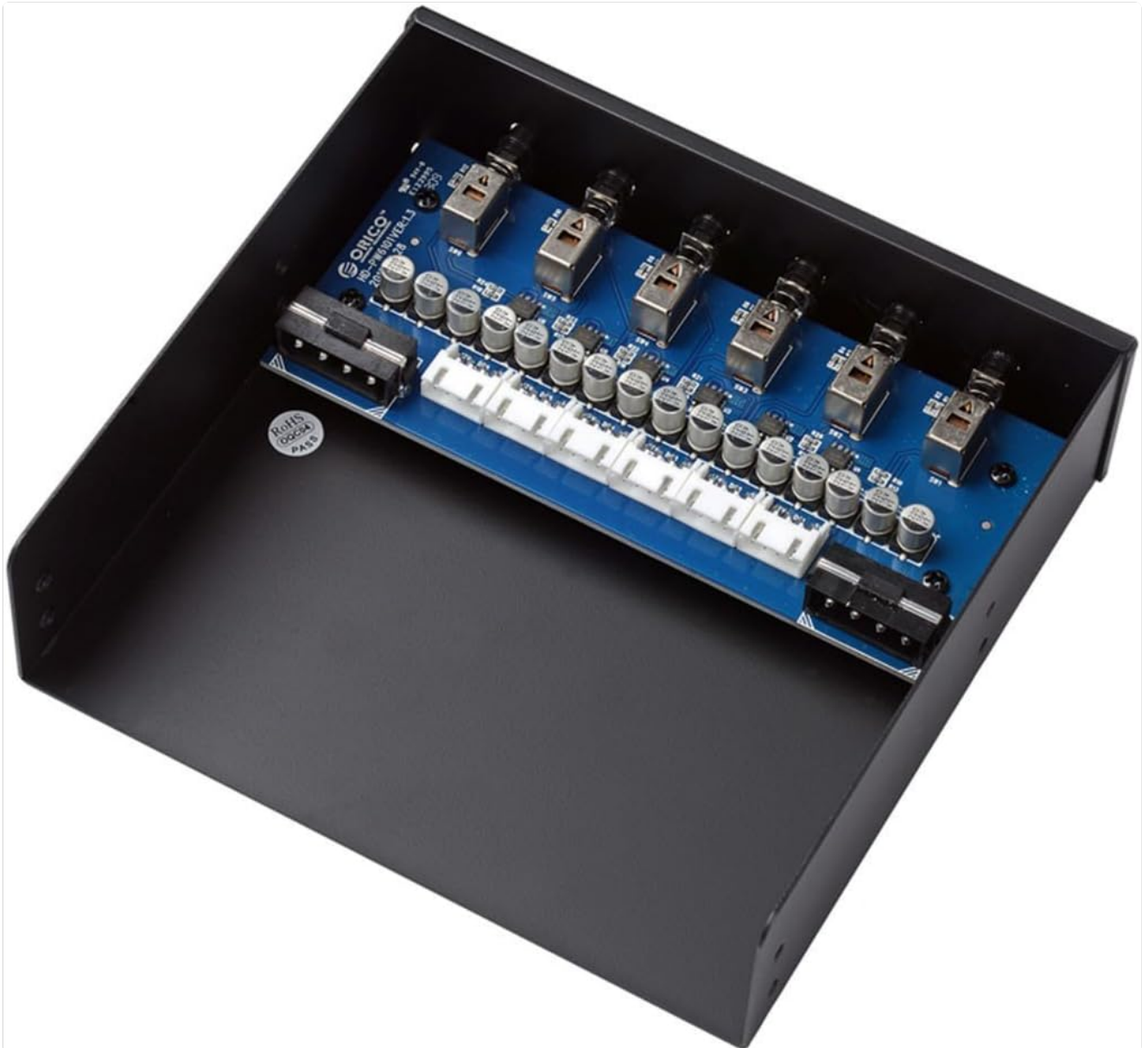
Figure 3: ORICO HD-PW6101 showing mounting points.
