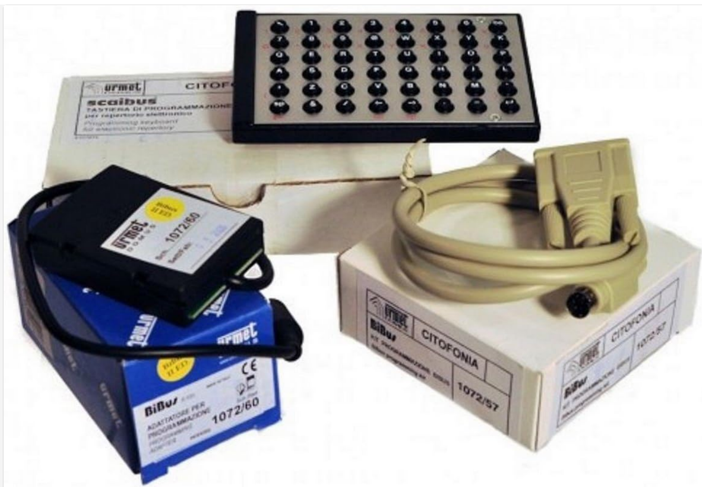
Figure 2.1: URMET BIBUS Programming Kit 1072/58 components. The image displays the programming keyboard at the top, the 1072/60 adapter module in its blue box on the left, and the 1072/57 connection cable with its box on the right.
