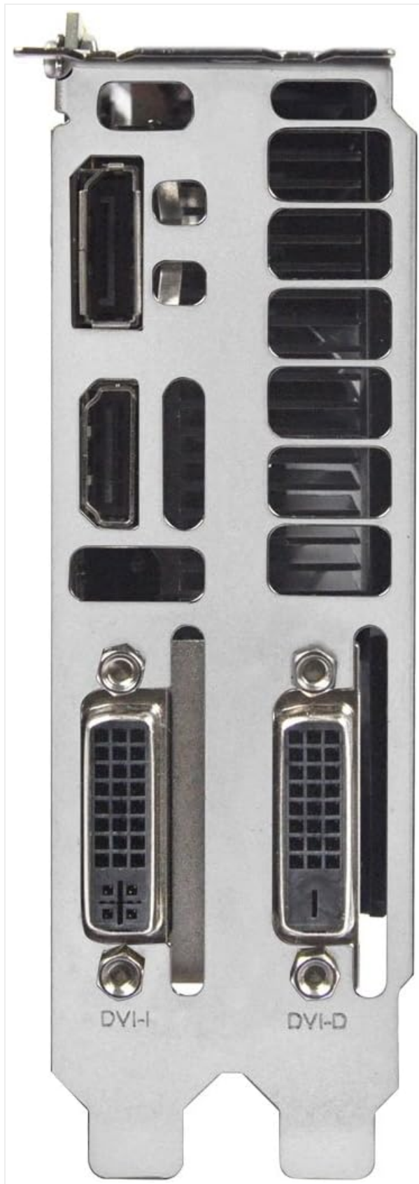
Figure 4: Display output ports on the graphics card, including DVI-I, DVI-D, HDMI, and DisplayPort.
