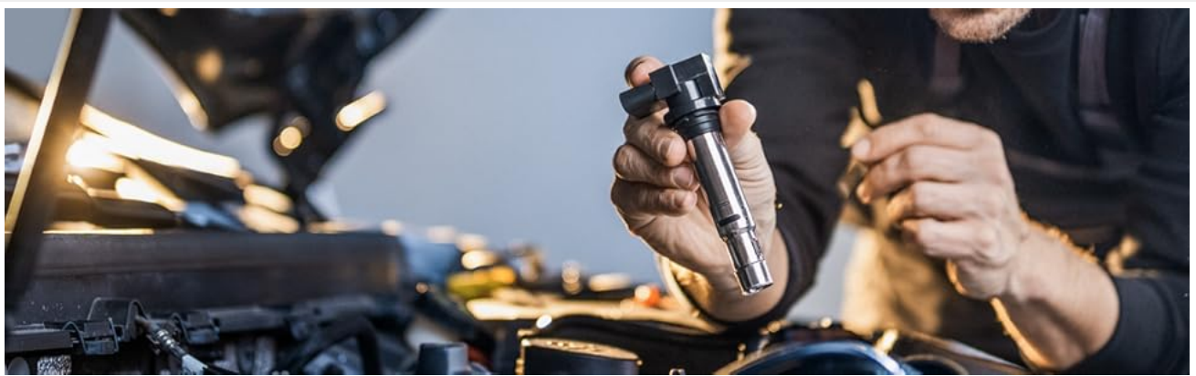
Figure 5.1: A mechanic inspecting an ignition coil. Regular checks are vital for identifying wear and ensuring proper function.
