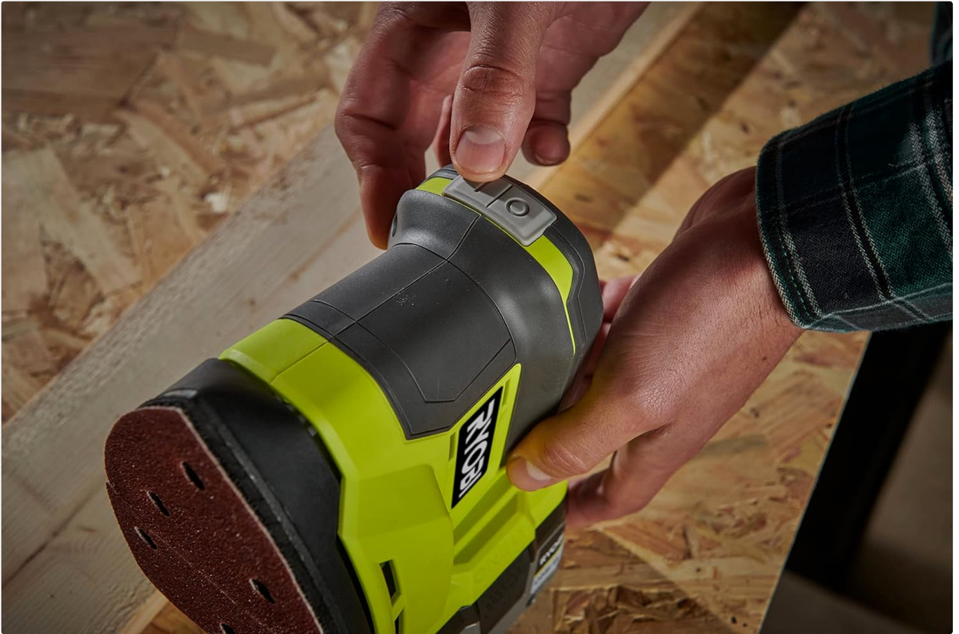
Figure 3: Using the triangular sander with an abrasive sheet on a wooden bench.
