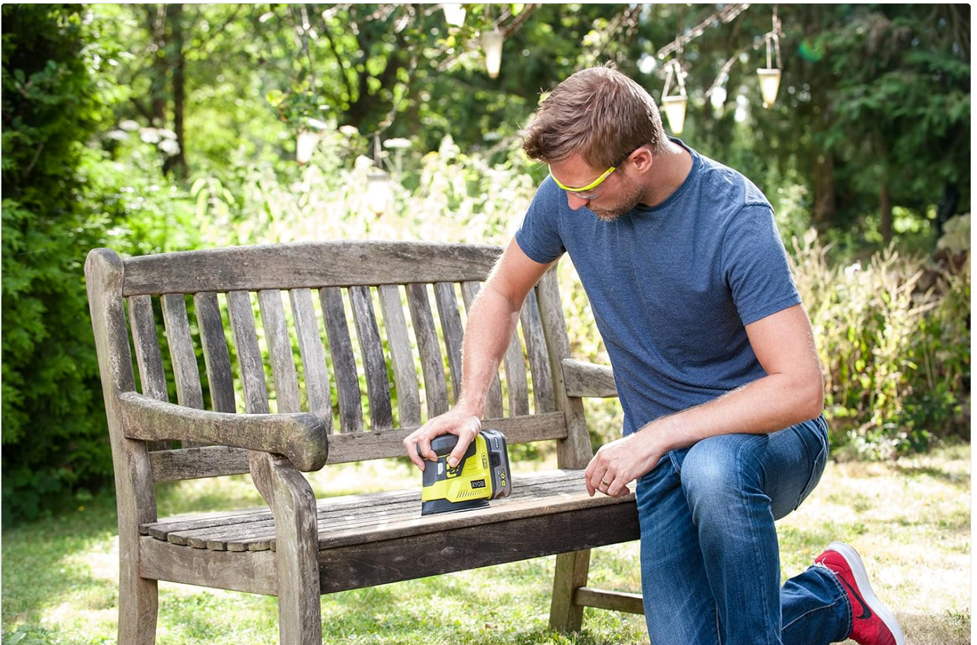
Figure 4: Sanding a wooden chair to prepare it for finishing.
