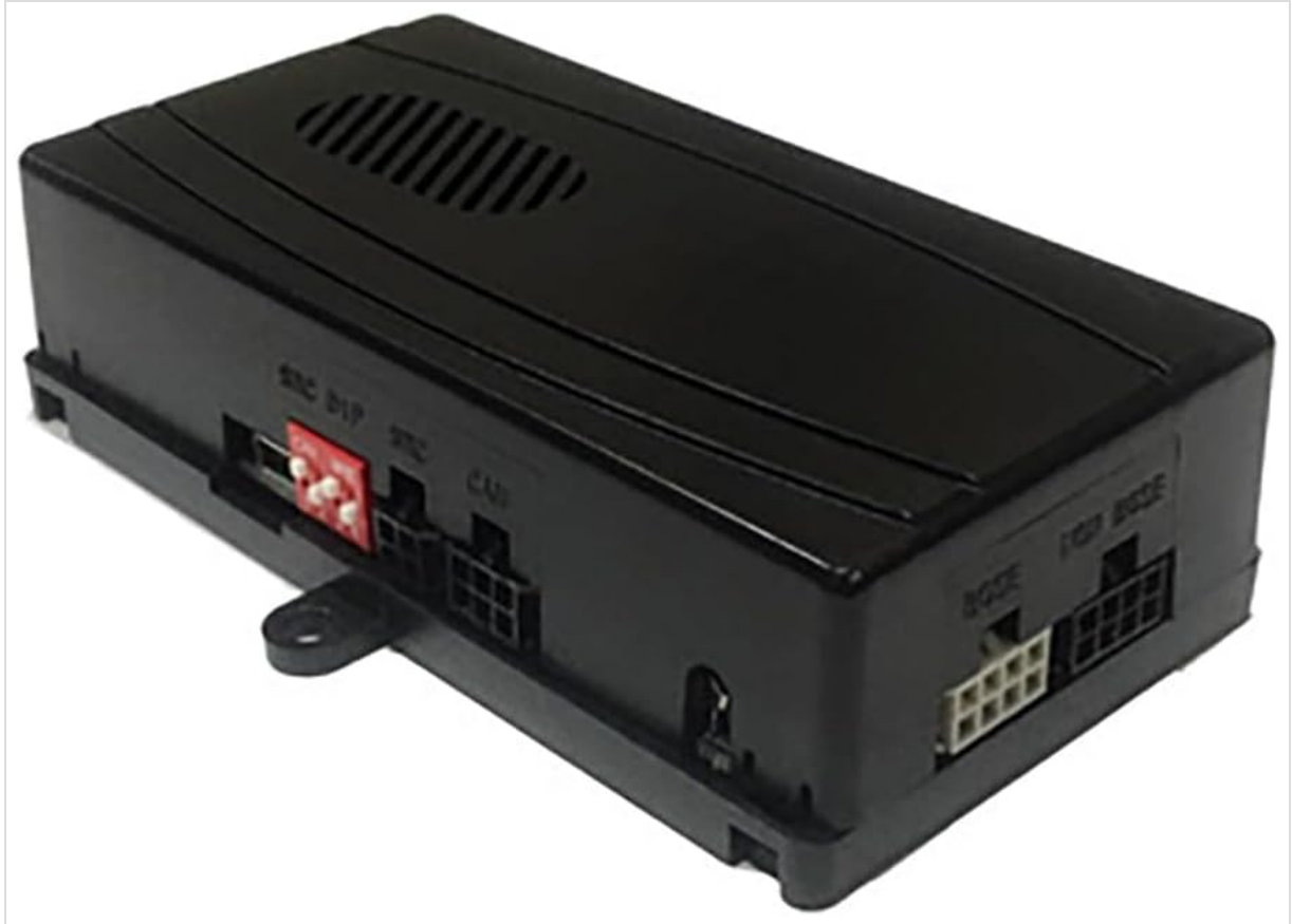
Image 3: A close-up view of the CRUX SOOGM-16 interface module, highlighting the dip switches. These switches must be set correctly according to your vehicle's configuration and aftermarket radio type.
