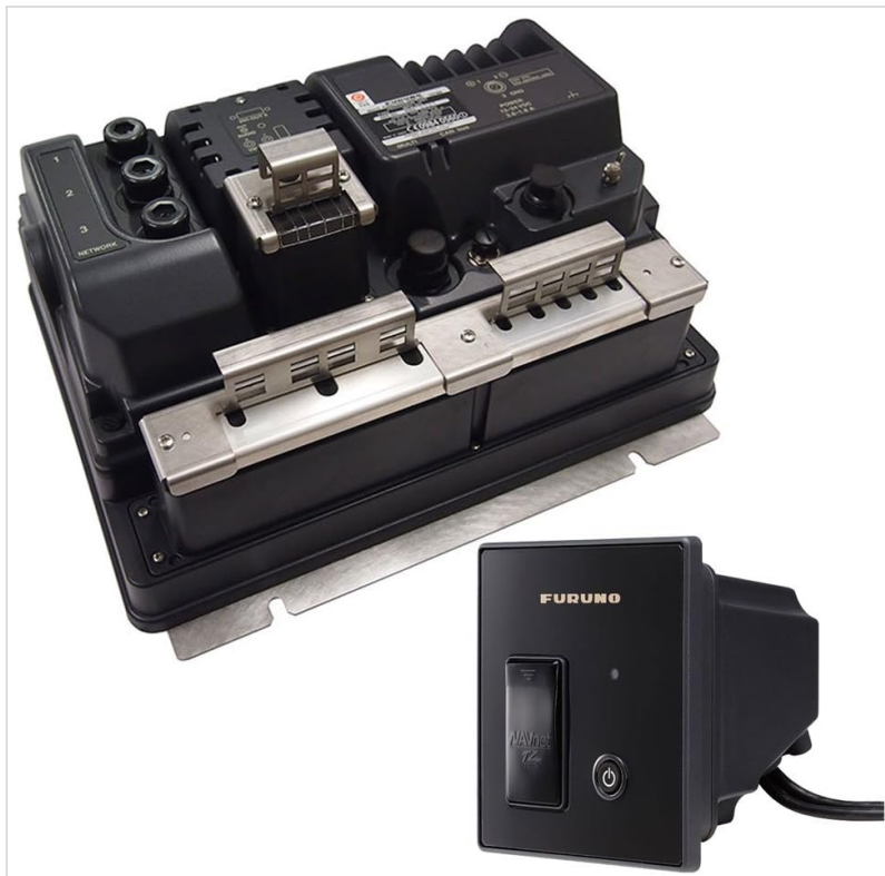
Figure 1: Furuno NavNet TZTouch Black Box with external power switch.
