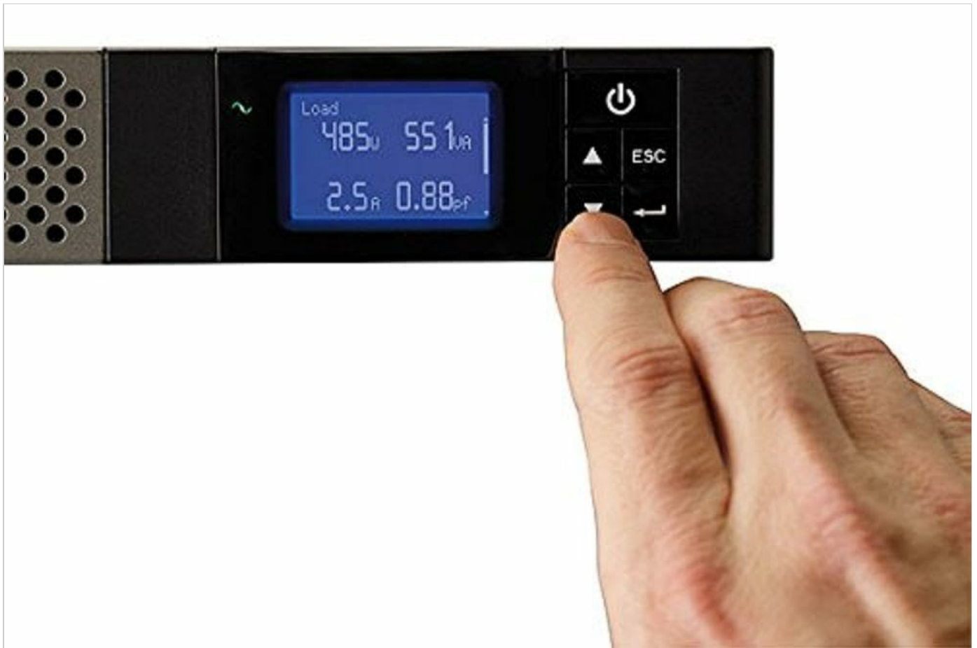
Figure 4.3: A hand interacting with the control buttons next to the LCD display on the Eaton 5P 1150i UPS. The display shows "Load" with values for voltage (485V), current (55.1A), and power factor (0.88pf). The buttons include Power, Up, Down, and ESC.
