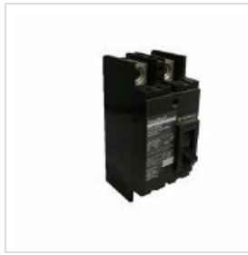
Figure 1: Front view of the Schneider Electric PowerPact QD 225 Circuit Breaker (Model QDP22225TM). The label clearly indicates "PowerPact QD 225 Circuit Breaker" and the model number "QDP22225TM". It also shows interrupting ratings for 240V at 25kA and 240V 1-phase at 10kA, suitable for 50/60Hz. The breaker features a toggle switch with "ON" and "OFF" positions and a red trip indicator. Terminal specifications for Al/Cu wires (#4 AWG-300 kcmil) are also visible, with torque settings of 75 lb-in (9 N-m) for the main terminals and 28 N-m for the smaller terminals.
