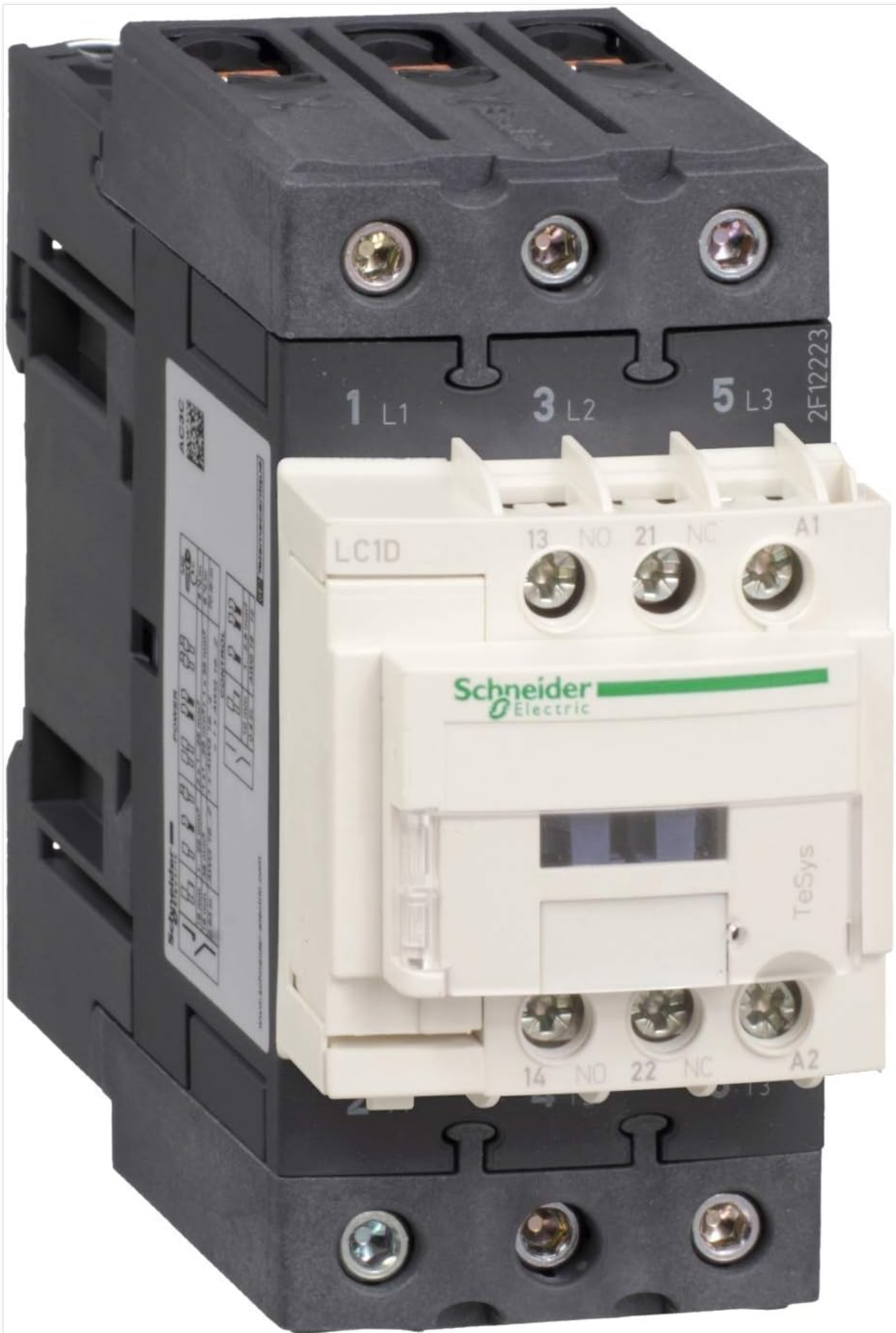
Figure 1: Schneider Electric TeSys D 3P Everlink AC Contactor LC1D50AM7. This image shows the front and side view of the contactor, highlighting the main power terminals (1 L1, 3 L2, 5 L3 at the top, and corresponding output terminals at the bottom), auxiliary contacts (13 NO, 21 NC, 14 NO, 22 NC), and the coil terminals (A1, A2). The Schneider Electric logo and TeSys branding are visible on the front face.
