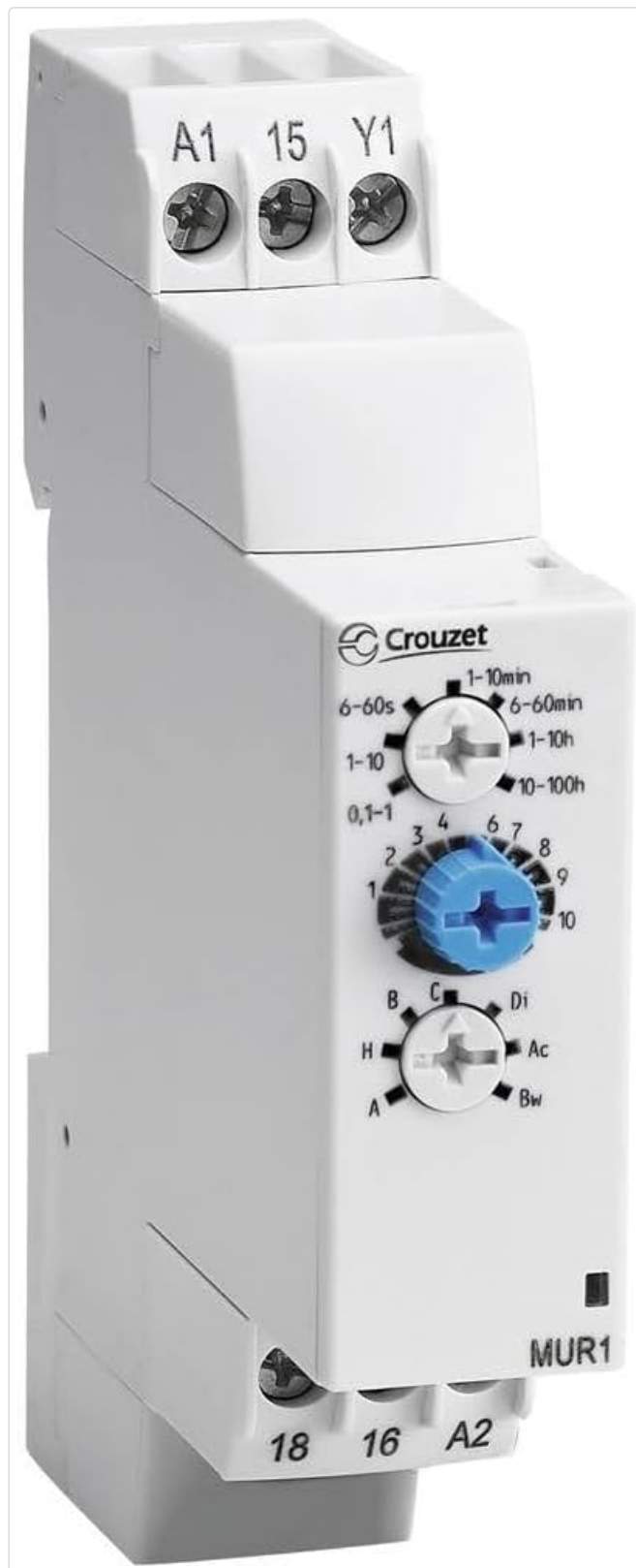
Figure 1: Front view of the Crouzet MUR1 multifunction timer, showing the control dials for time range, timing value, and function selection, along with terminal connections.
