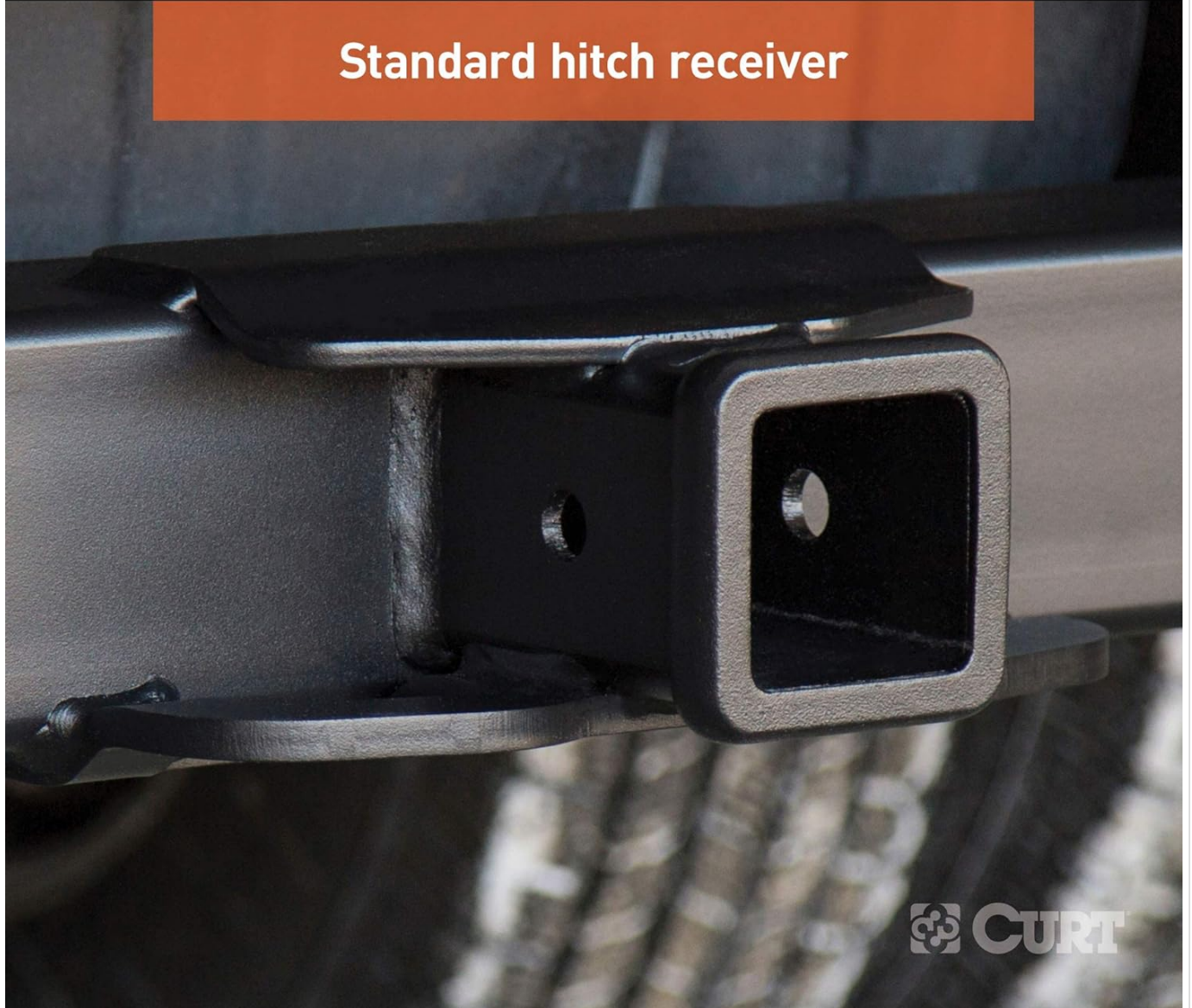
Figure 3: A close-up view of the 2-1/2 inch standard hitch receiver, designed to accommodate heavy-duty towing accessories.
