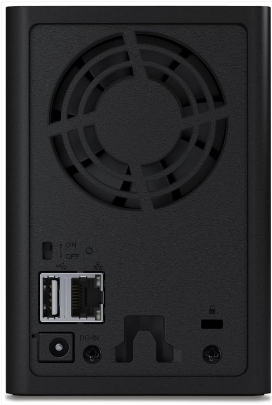
Figure 2: Rear panel of the LinkStation 420, showing Ethernet, USB, and power ports.
