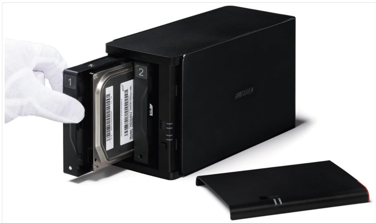
Figure 5: Illustrative view of hard drive insertion into the LinkStation 420.
