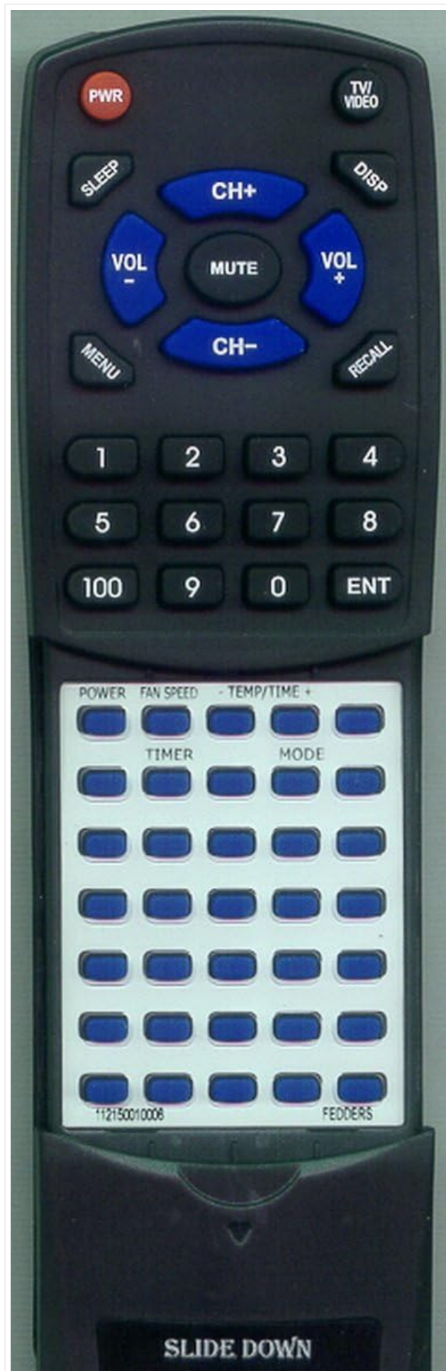
Figure 1: Front view of the Redi-Remote Replacement Remote Control. The remote features a top section with primary controls like power, channel, volume, and number pad, and a lower section with additional function buttons hidden under a sliding cover.
