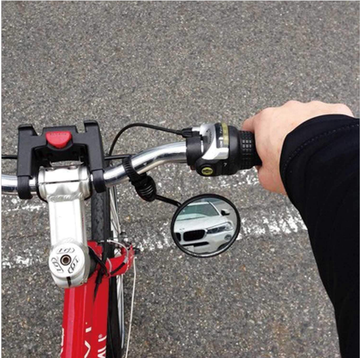
Figure 4: Example of the view provided by the Cycle Star 80 mirror. The convex lens offers a wide perspective, allowing the rider to see approaching vehicles and other elements in their rearward path.
