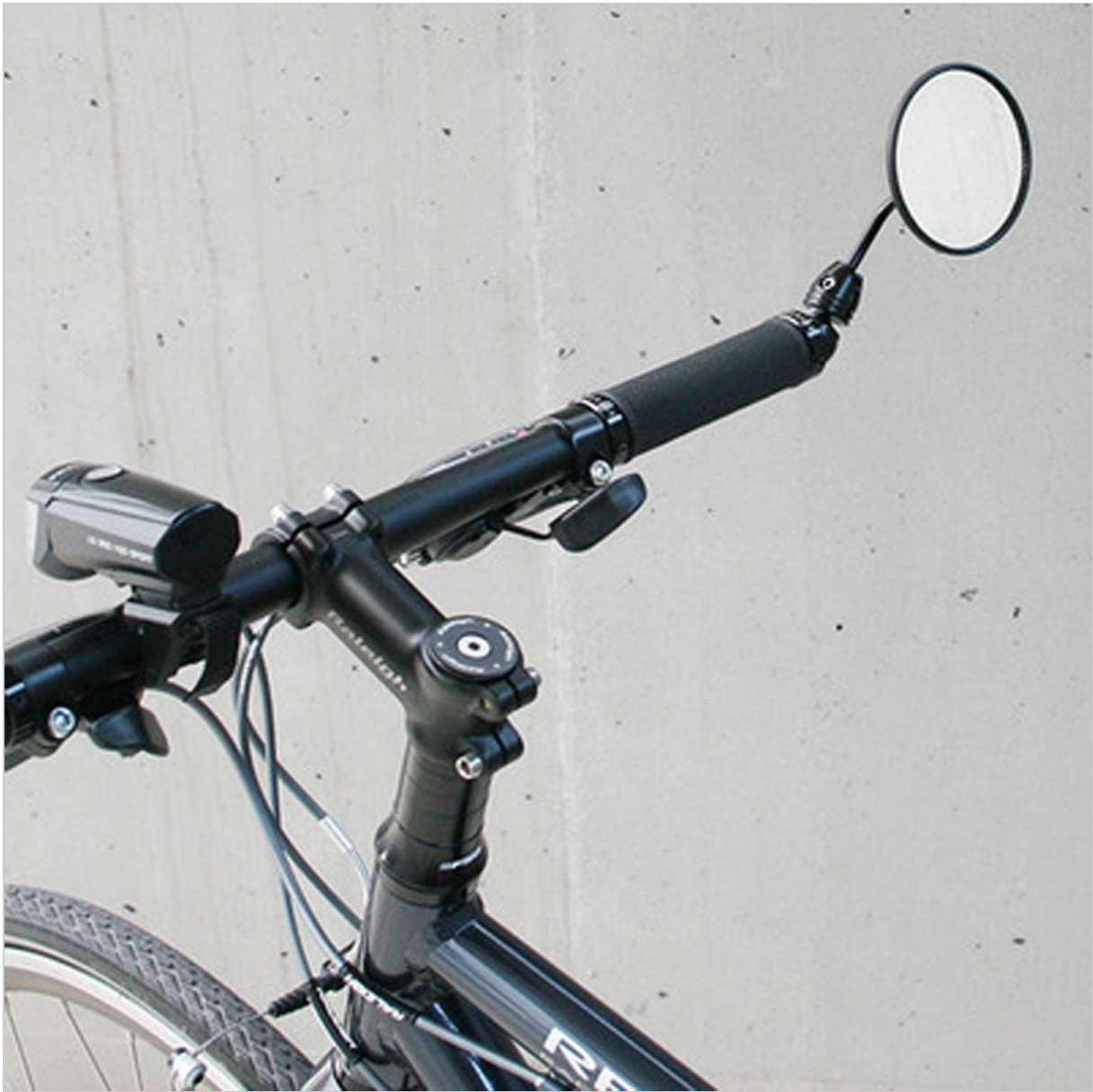
Figure 3: Front view of the mirror installed on a bicycle. The mirror's position can be adjusted to optimize the rider's rearward visibility, ensuring it does not interfere with hand placement or controls.
