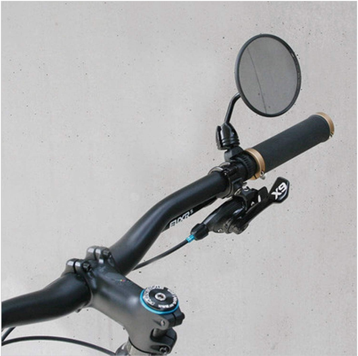
Figure 2: Side view of the mirror mounted on a bicycle handlebar. The short arm allows for a compact installation, typically near the handlebar grip or brake lever, providing a clear rear view without excessive protrusion.
