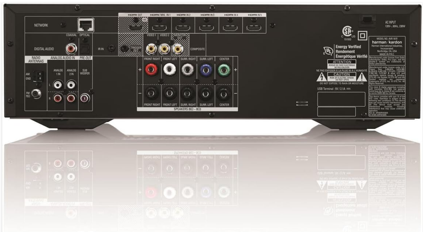
Figure 1.2: Rear panel of the Harman Kardon AVR 1610, illustrating speaker terminals, HDMI, and other audio/video inputs.
