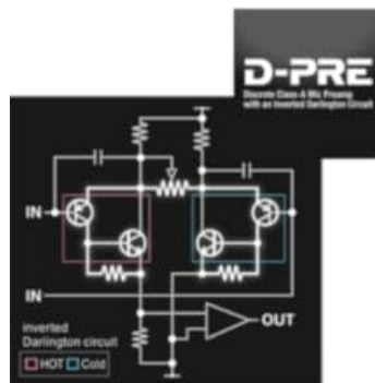
Image: Diagram illustrating the D-PRE Discrete Class-A Mic Preamp circuit with an inverted Darlington design.
