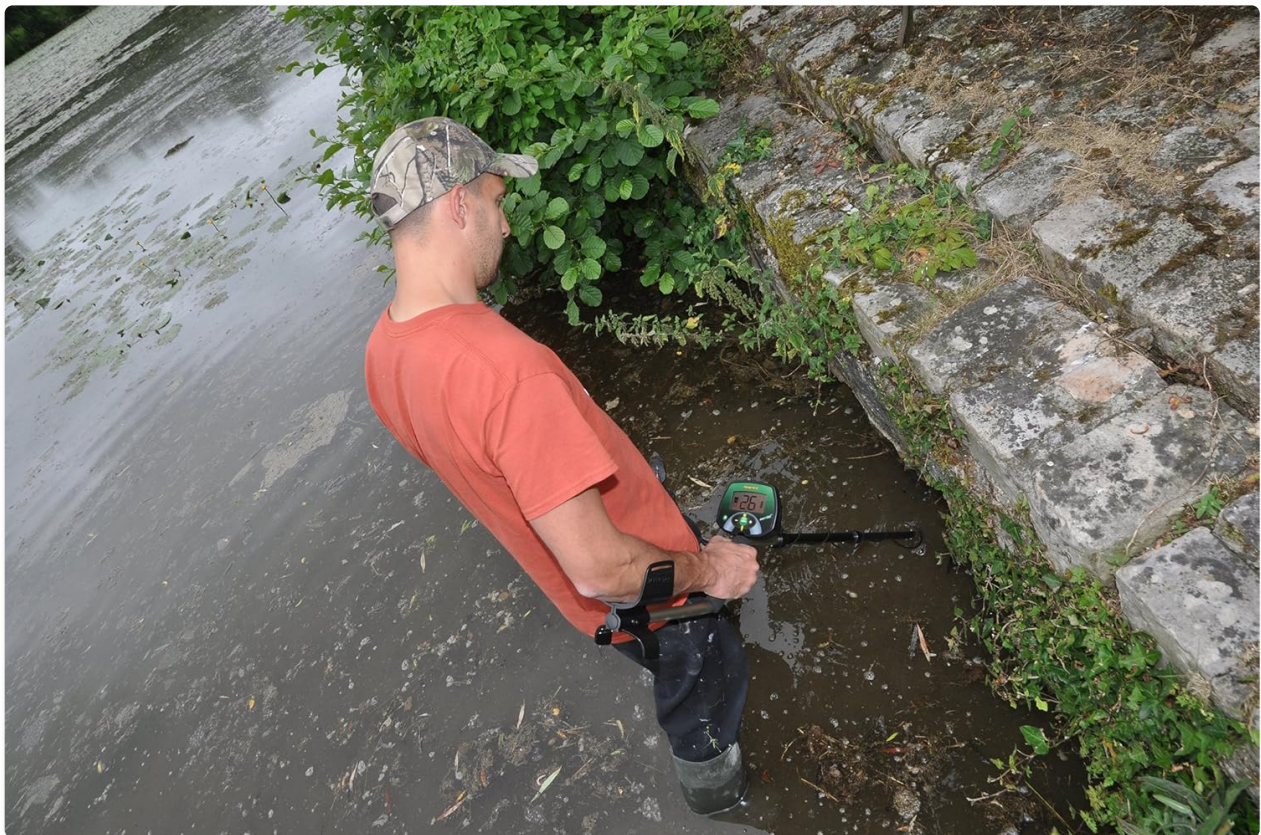
Figure 3: The waterproof search coil allows for detection in shallow water.
