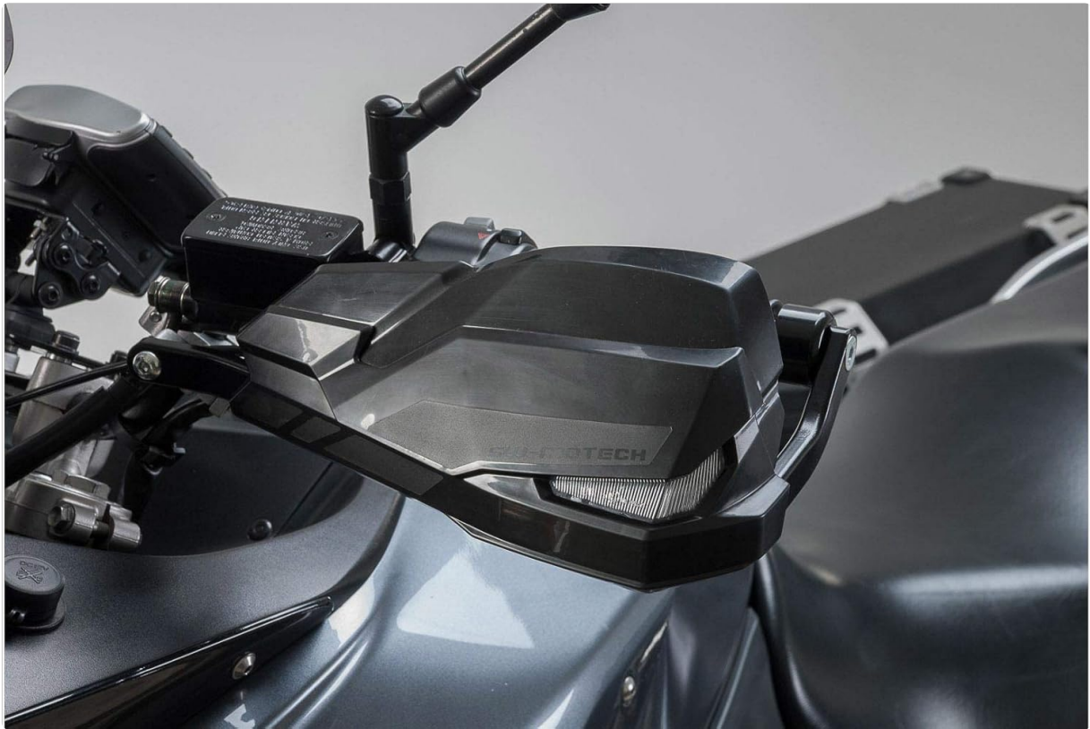
Image 1: SW-MOTEC Kobra Handguard Kit installed on a motorcycle. This image shows the handguard mounted on the handlebar, providing protection for the rider's hands and controls, with the SW-Motech logo visible.
