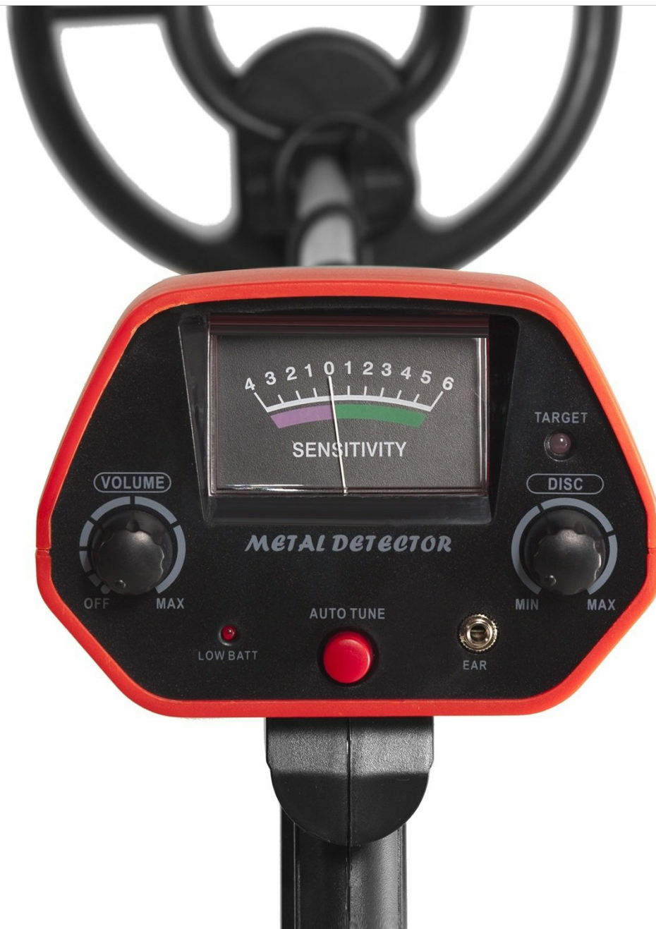
Figure 2: Detailed front view of the control panel, highlighting the 'SENSITIVITY' meter, 'VOLUME' and 'DISC' knobs, 'AUTO TUNE' button, 'LOW BATT' indicator, and 'EAR' (headphone) jack.
