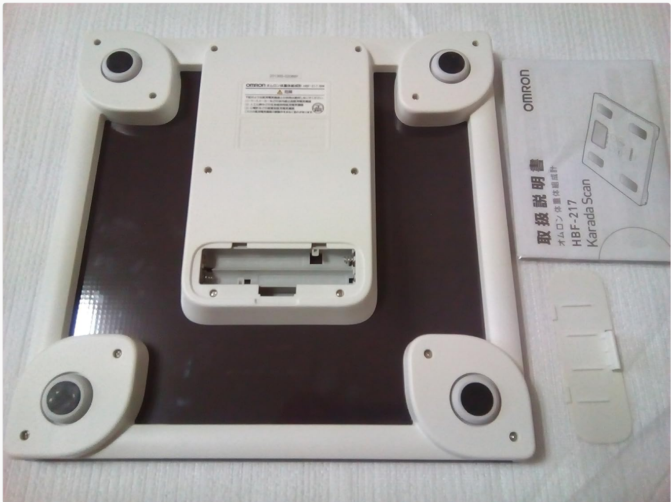
Image: The underside of the OMRON HBF-217-BW Body Composition Monitor, showing the battery compartment and the included instruction manual.
