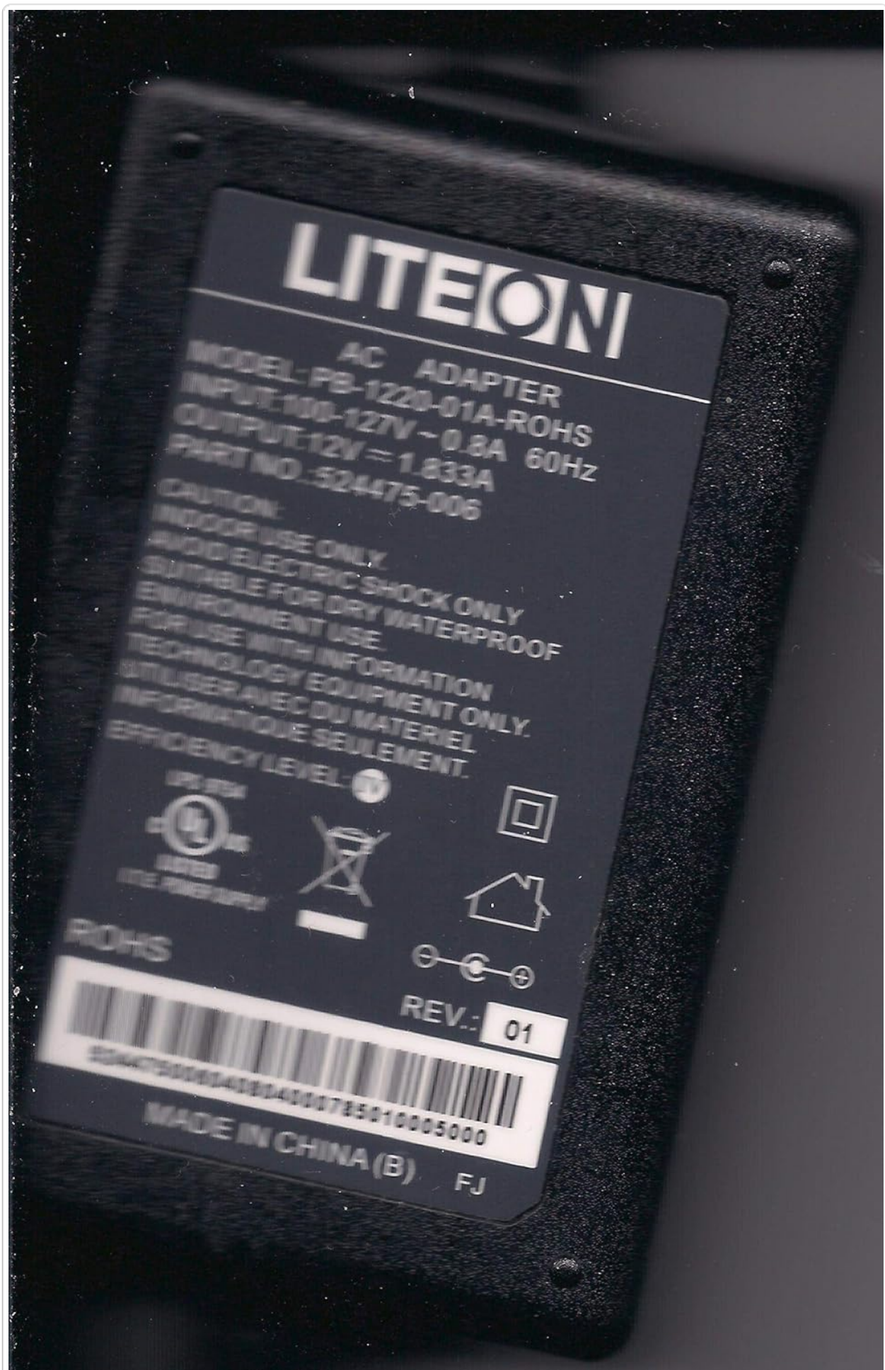
This image displays the LiteOn PB-1220-01A-ROHS AC Adapter. The label on the adapter clearly shows the model number, input and output electrical specifications, part number, and various safety certifications and warnings. The text 'MADE IN CHINA (B)' and 'REV.: 01' are also visible.
