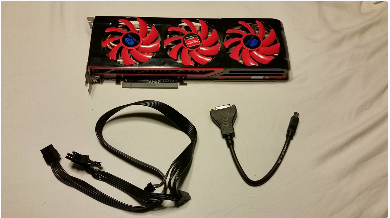
Image: Top view of the Sapphire Radeon HD 7990 graphics card, showing the three cooling fans and the heatsink assembly. The card features a black and red design.
