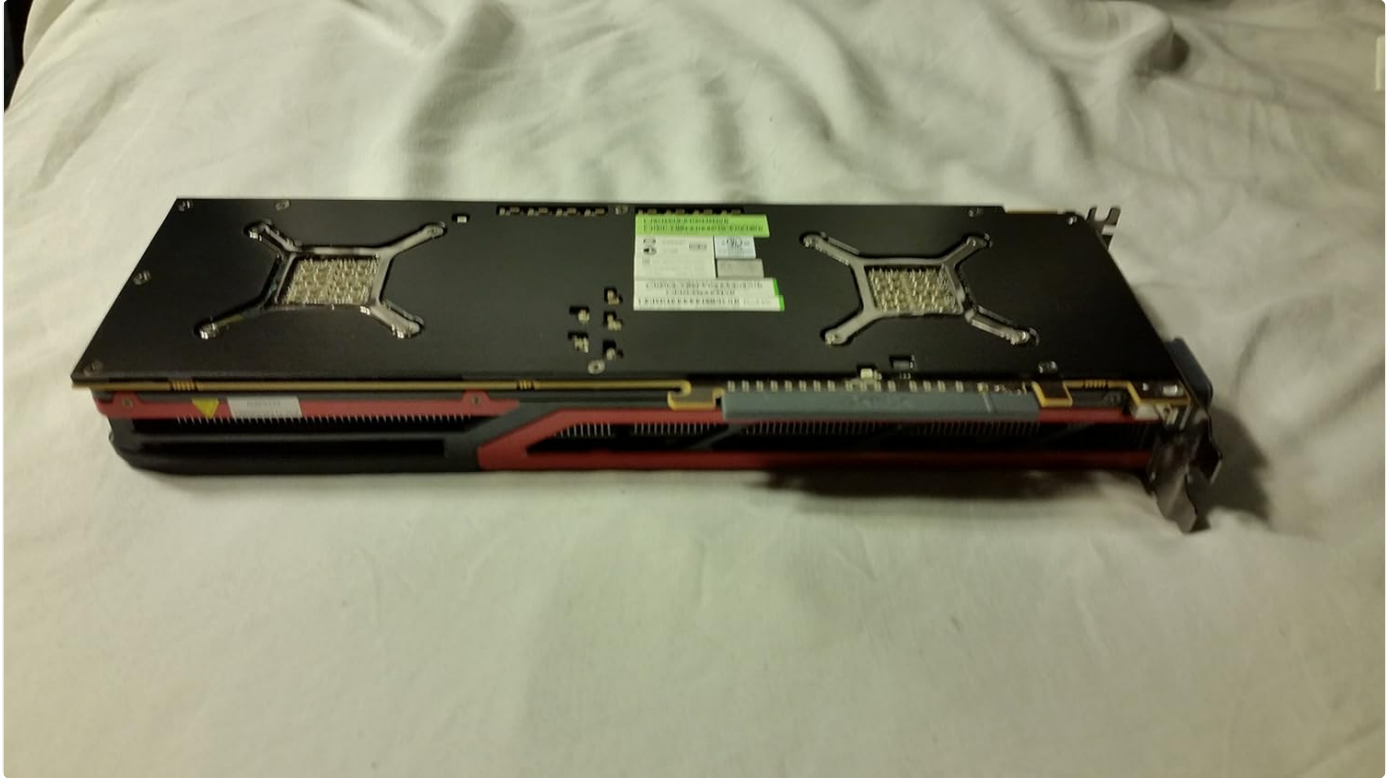
Image: Backplate view of the Sapphire Radeon HD 7990 graphics card, showing the PCB and mounting points for the cooler.
