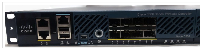
Figure 2: Front panel of the Cisco 5508 Controller, showing network ports (Gigabit Ethernet and SFP), USB ports, console port, and status LEDs.
