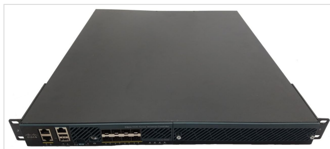
Figure 1: Top-down view of the Cisco 5508 Series Wireless LAN Controller, showcasing its compact rack-mountable form factor.
