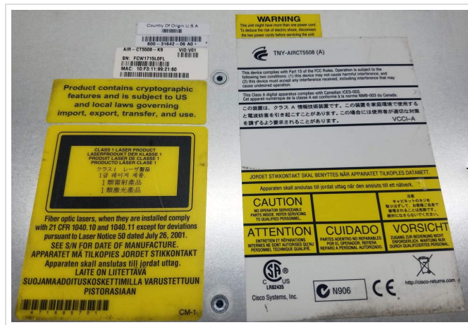
Figure 6: Various regulatory and warning labels found on the Cisco 5508 Controller, including FCC compliance and laser safety information.
