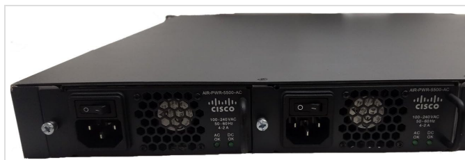
Figure 4: Detailed view of the AC power supply units (AIR-PWR-5500-AC) for the Cisco 5508 Controller, showing power inputs and status indicators.
