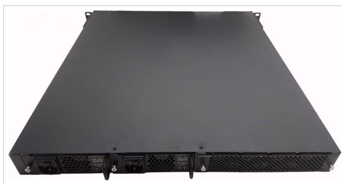
Figure 3: Rear view of the Cisco 5508 Controller, highlighting the bays for redundant power supply units.
