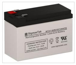
Image: SigmasTek SP12-7.5HR (12V 7.5Ah) Sealed Lead-Acid Battery. The label displays the brand name, model number, battery type, charging instructions (Floating use: 13.5-13.8V, Cycle use: 14.4-15.0V, Initial current: less than 2.1A), and recycling symbols including a 'Pb' for lead, and a crossed-out waste bin indicating separate disposal. UL recognition mark MH47929 is also visible.
